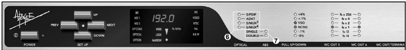
**6) OPTICAL** – This parameter determines the format of the Optical Input/Output connectors.
