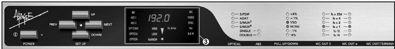
**3) CLOCK /Digital Audio SOURCE** – At it’s simplest, Big Ben derives a reference clock frequency from an internal or external source and generates several ultra low jitter clock outputs based on this reference. The CLOCK SOURCE parameter selects the source of the reference clock frequency. When a Clock Source is selected which contains a digital audio signal, that signal is routed to all outputs capable of transmitting digital audio. The following sources are available:
